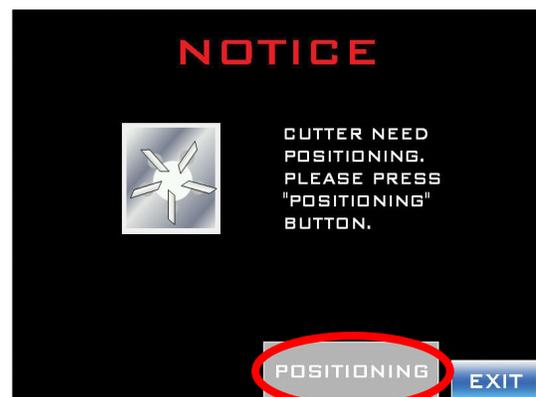
4. Press the “Positioning” Button. The Cutter Blades will rotate into their home position. The system is now ready for the label film to be installed.
