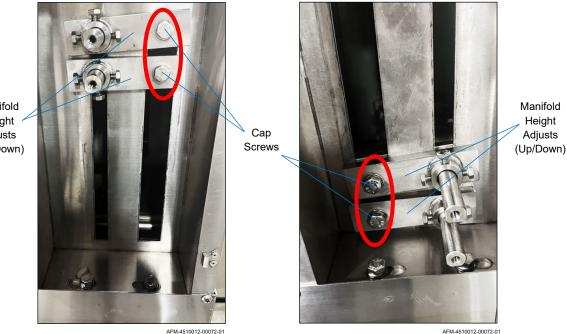
Manifold Height Adjusts (Up/Down) 4. Adjust the height of the Upper and/or Lower Manifolds as desired. The Manifolds do not need to remain parallel to one another. Maximum height variation for a single Manifold is 7.5" (19.1 cm).
